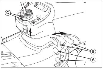
Figure 3. Engaging the Parking Brake
